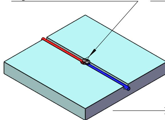
Drill the hole of 12mm diameter and 57-60mm depth
