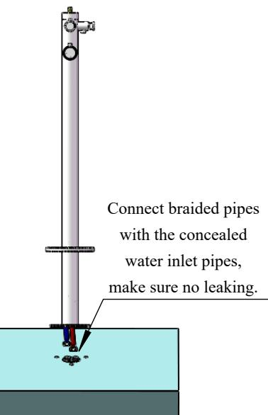
Connect braided pipes with the concealed water inlet pipes, make sure no leaking.
