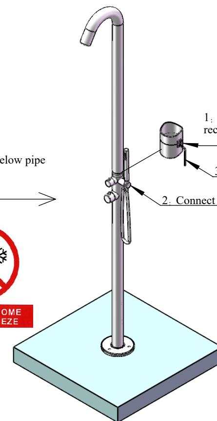
1. Match the back line together with two pipes, make sure in rectangle, and lock the fixing screw.
